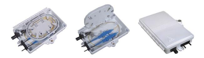
Fiber Optical Terminal Box is used in the end termination of residential building and villa, to fix and splice with Pigtails or connected fast connectors can be installed on the outside wall. For connecting up to 12 LC or 6 SC connectors. In order to prevent access by unauthorized people, the box door is equipped with a lock and key. In addition, the box can be sealed.
